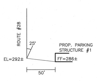
ANGLE OF BULK PLANE DIAGRAM
